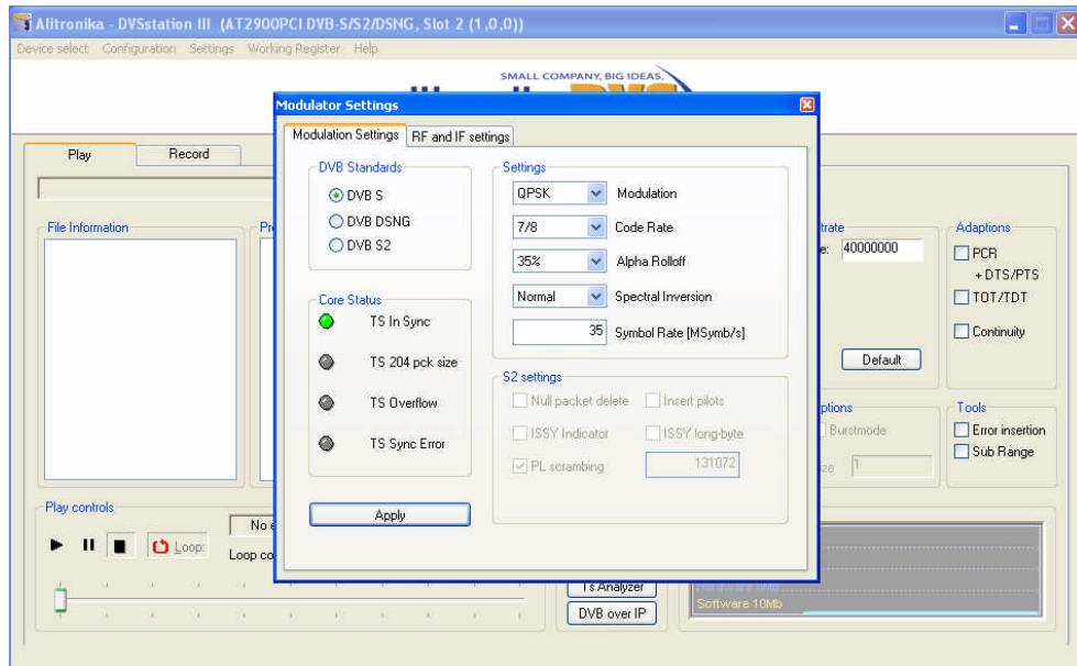
The IF & RF setting options are common for all Alitronika modulators. The frequency range, output level range and IF frequencies differ according to DVB standards & modulation schemes. For example for DVB-S/S2 modulators the selectable frequency range is 950-2150MHz. The IF frequency is selectable between 49-51MHz or 99-101MHz.
