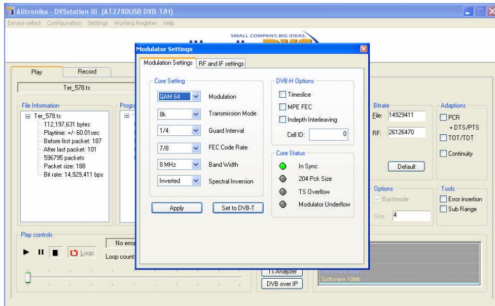
The Screen shot below shows the modulator parameter settings for DVB-C modulators. There are annexes A, B and C. The extended QAM256 mode can be selected in DVB C Option. A “Free Mode” allows the user to select parameters outside J83 standards.
