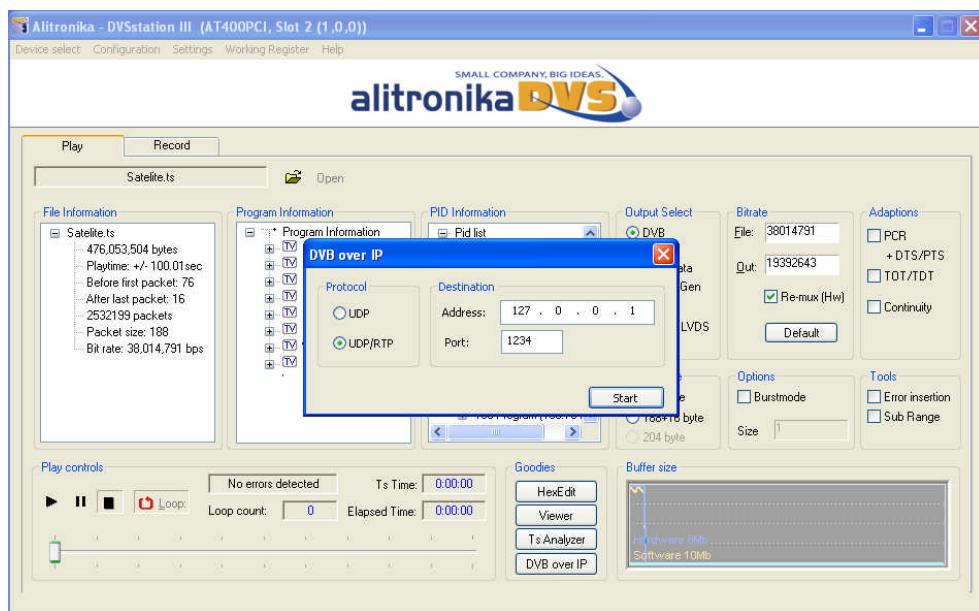
The resulting DVB-IP stream could be received, recorded, viewed & analyzed by an instant of DVSStation3 or VideoLan running on a remote PC/Laptop on the same network.
