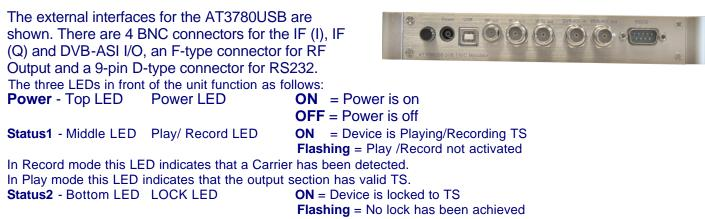
In Record mode this LED indicates that the device has locked into incoming TS. In Play mode this LED indicates that the output section has locked into outgoing TS.
