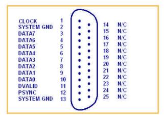
LVTTL/LVCMOS input & output Pinout
