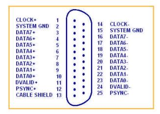
LVDS input & output Pinout
